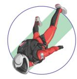
After the skydiver releases his parachute, the shape and area has been changed and so the amount of air resistance acting is increased. This causes him to decelerate and his terminal velocity is reduced to about 15mph. This makes it a much safer speed to land on the ground.
