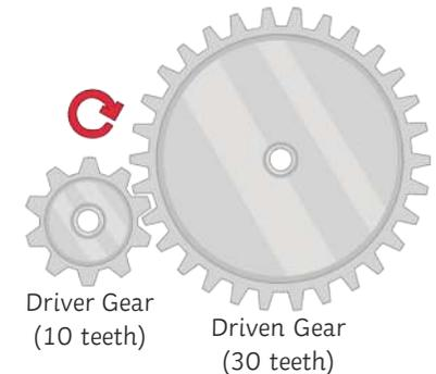
When gears are connected, the **same force** is applied to each; however, if they are different sizes, they will produce **different moments**. This is because the moment is calculated using the distance from the pivot (the radius of the gear) and if the gear is smaller, it will move a shorter distance. If the gear is larger, it will move a greater distance.
