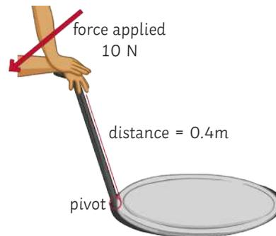
A force multiplier makes it easier to do work because the same force applied at a greater distance from the pivot increases the moment produced.
